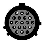
Wiring details for the compatible socket, \*\*\*-14-19S, as seen from the cable end.
