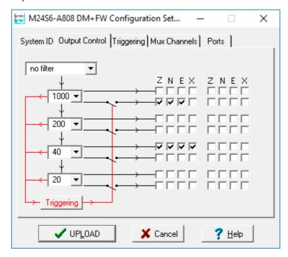
With this configuration uploaded, Tap 2 will continue to produce output at all times, but Tap 0 will also emit data whenever the trigger criteria are met. The *Triggering* button is now shown in red to remind you that the trigger is active.
