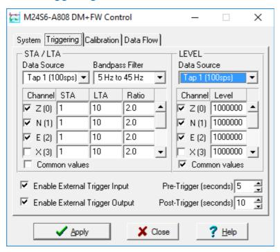
The *Triggering* pane is very similar to the corresponding pane of the *Configuration setup* window ( see section 5.1.3 page 38), although not all of the options described there are available here, since some require rebooting the digitiser.
