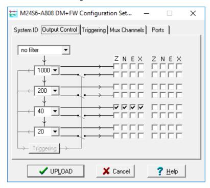
Güralp digitisers initially sample incoming data at a high rate (e.g. 2000 Hz for the DM24), which are then filtered and reduced to a lower rate (decimated) using an on-board digital signal processing unit, or DSP. The DSP has several filtering/decimation stages, which run one after the other. Stages which can produce output are called *taps*. The Güralp DM24 can output 4 taps simultaneously.
