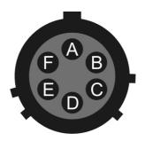
Wiring details for the compatible socket, \*\*\*-10-06S, as seen from the cable end.
