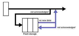
Instructs the DM24 to transmit current blocks to clients if possible, but to store all unacknowledged blocks in the Flash memory and re-send them, oldest first, when time allows. *ADAPTIVE* mode is best suited for "real-time" installations where the link between digitiser and client is intermittent or difficult of access.
