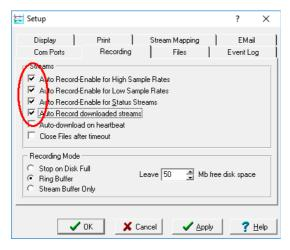
Ensure that the first four check-boxes are ticked. Next, switch to the "Files" tab and choose an appropriate base directory, file format and filename format.
