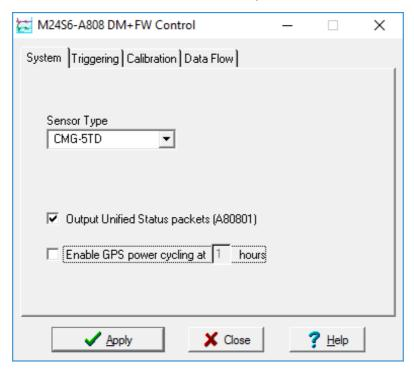
**Sensor Type:** If the sensor attached to the digitiser is a Güralp velocity sensor, you can send control commands to it from the *Mass Control* tab (see below). Which functions are available on this tab depends on the *Sensor Type* you have set here.
