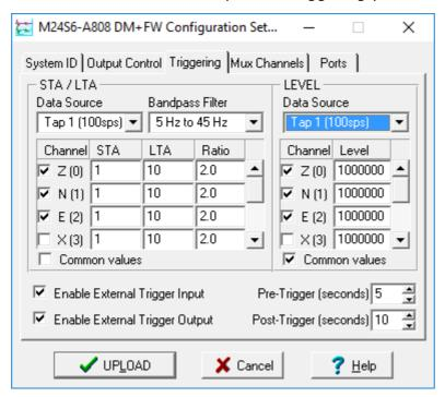
There are two triggering algorithms which Güralp digitisers can use. However, not all models can use both methods. Scream! will interrogate the digitiser to discover which methods are supported by its on-board software.
