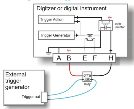
To trigger an instrument from an external source through a relay:
