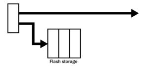
Instructs the DM24 to transmit streams directly to clients as for *DIRECT* mode, but also to store all data into Flash storage as for *FILING* mode.
