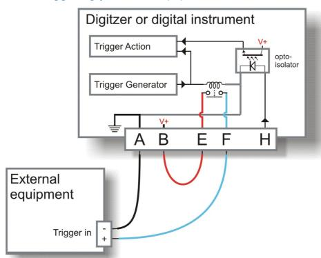
If your equipment can trigger from 24 V DC, the simplest arrangement is to use the voltage across the sensor's power supply as a trigger.
