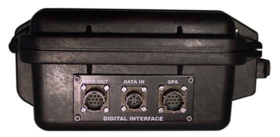
The DM24 transmits data through its DATA OUT port. This is an RS232-compatible serial link, outputting data in GCF format according to the particular configuration of the instrument. The DM24 has a default baud rate of 38,400. You can change this from the command line using the BAUD command or from Güralp Systems' control, acquisition and monitoring software package, Scream! (see Chapter 5 on page 33).
