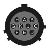
Wiring details for the compatible socket, \*\*\*-12-10S, as seen from the cable end.
