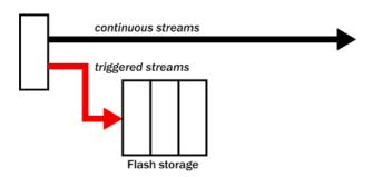
Instructs the DM24 to transmit any *continuous* streams directly to clients as for *DIRECT* mode, but to store *triggered* data into Flash storage as in *FILING* mode.
