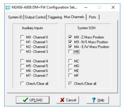
If a tick is placed in the box next to a channel, its data will be collected and transmitted as a data stream in GCF format, just as with the normal data channels. To indicate that the data come from a Mux channel, the Stream ID will take the form \*\*\*\* $M_{\underline{X}}$ , where M stands for Mux and  $\underline{X}$  is a hexadecimal integer (*i.e.* 0 – 9, and A – A for 10 through 15). A A and A respectively.
