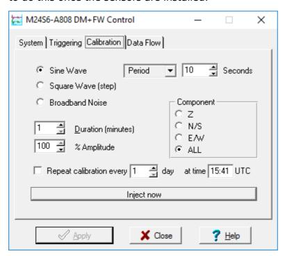
Each channel **Z, N/S** and **E/W** can be calibrated separately. For most triaxial digital instruments, each channel calibrates the corresponding axis of the instrument; simply select one of the **Z, N/S** and **E/W** check boxes to calibrate that axis. Some instruments use only one calibration loop, which is reproduced for all three components: if you have one of these instruments, you should select **Z** to calibrate the sensor.
