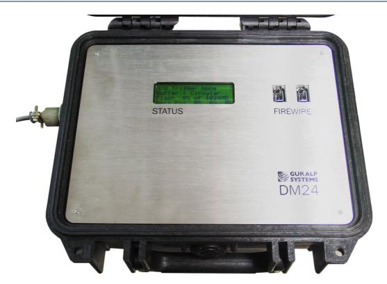
Before you can use the disk, you will need to reset it. The DM24 saves data on the hard disk in a special format, DFD, so you *cannot* use your PC's operating system tools to reset the disk.
