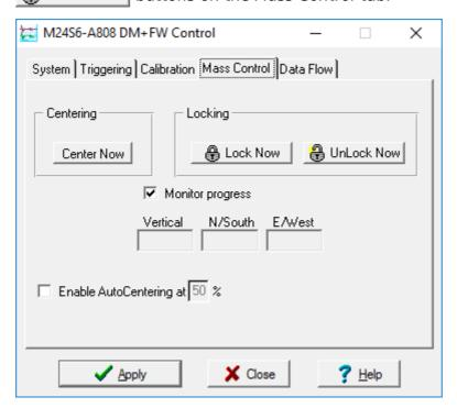
If you select **Monitor progress**, the window will remain open during the process, and the mass positions will be displayed in the Vertical, N/South and E/West boxes. If you leave **Monitor progress** unselected, the window will close. You can still monitor mass positions by selecting the appropriate streams and opening a WaveView window for them.
