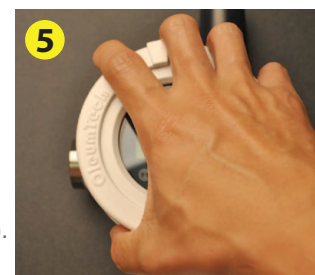
Tighten the enclosure cover by hand only.
