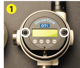
Remove the enclosure cover and detach the LCD Module secured by the screws.
