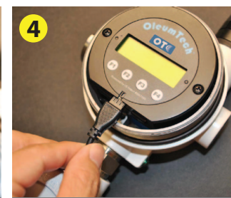
Program the transmitter using the PC or through the LCD interface.
