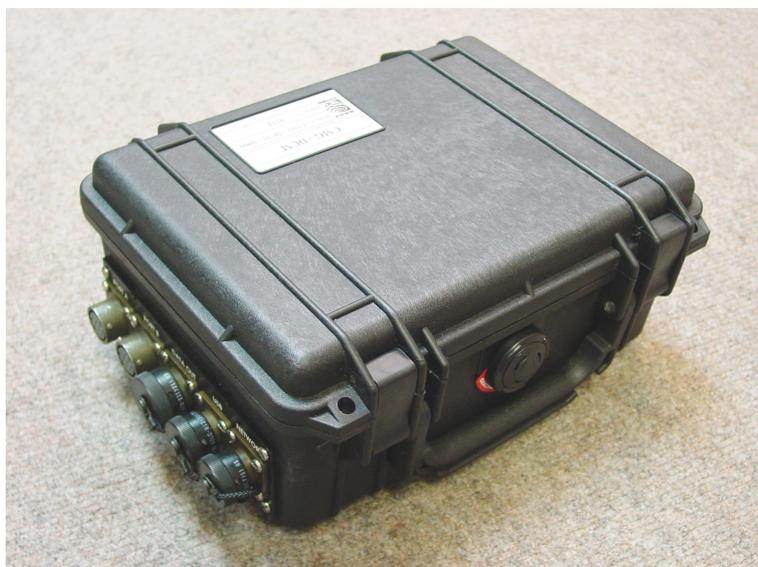
A stand-alone DCM unit is normally supplied with a high-capacity removable disk for data storage. These disks allow the DCM to be used as part of completely autonomous installation in cases where communications links are poor or non-existent. Manufactured and tested at Güralp Systems, the disks are compatible with USB and FireWire standards and include an internal temperature sensor and heater for use in cold environments.
