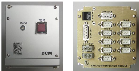
Up to four modules may be mounted side-by-side in a 19" rack.
