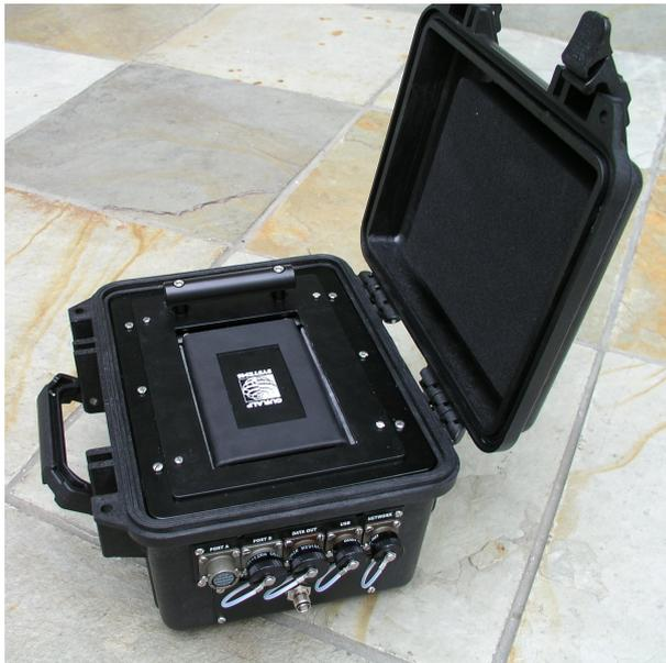
You can retrieve data from a DCM's disk at any time by removing it from the module and attaching it to a PC using a USB or FireWire cable. Swapping disks does not cause any risk to data.
