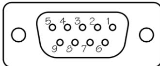
Wiring details for the compatible plug, DE9M, as seen from the cable end (i.e. during assembly).
