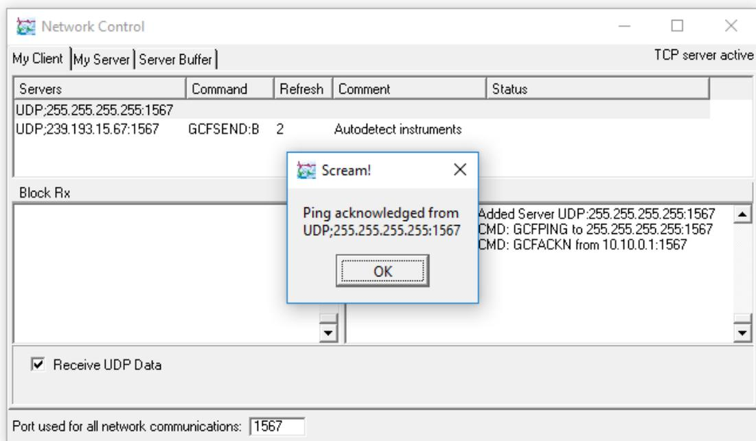
In this case, a single acknowledgement response (GCFACKN) was received and it came from the address 10.10.0.1 so this is the address of the NAM. If there are more than one NAM (or other GCF servers) on the network, multiple GCFACKN packets will be reported, as shown here:
