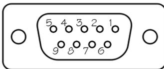
Wiring details for the compatible plug, DE9M, as seen from the cable end (i.e. during assembly).
