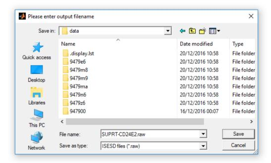
The extension must be given for the program to recognize in which data format to export the data. A file-name is automatically suggested by ART based on the name listed in the central list box. If the user has entered metadata concerning the earthquake and station associated with a time-history, this information is included within the exported files in agreement with the selected file format. This is a significant improvement with respect to previous versions of ART.
