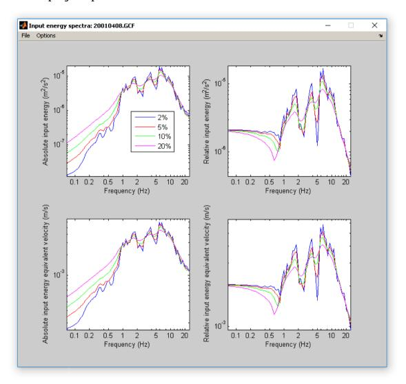
The undamped spectra are also computed but are not displayed due to their limited applicability in engineering seismology/earthquake engineering. The calculation takes a few seconds for a normal length time-history. The method given in Beaudet & Wolfson (1970) is used to calculate the spectra. The spectra are displayed using the units selected by the user in the 'Options' window and using the other selected options.
