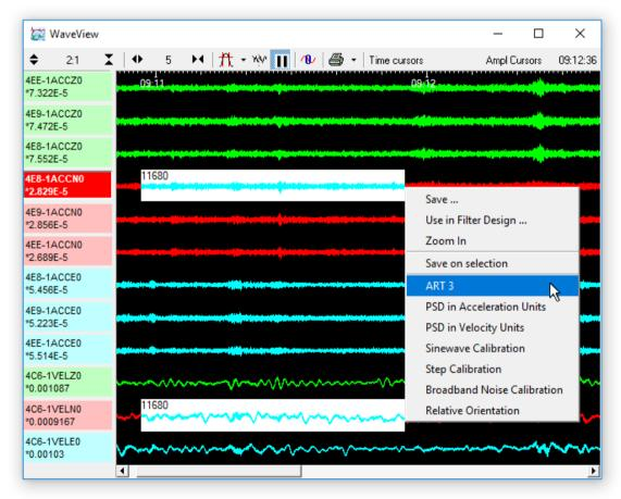
The second illustration shows the selection of two non-adjacent streams for comparison. To do this, hold down the Ctrl key and drag a box from the start-time on the first stream to the end time on the second stream.
