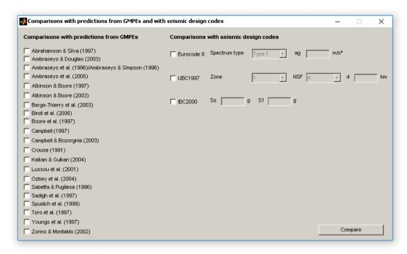
Once the user has selected the GMPEs and the codes to compare with the observed elastic response spectra for the selected time-histories (and, if a seismic design code has been selected, entered the necessary information), clicking on the Compare button opens a new window displaying the predicted and observed spectra (see below). The predicted spectra are referred to by the abbreviations given above.
