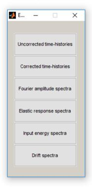
Clicking on this button opens up a window that enables the user to export uncorrected acceleration time-histories, corrected acceleration, velocity and displacement time-histories, Fourier amplitude spectra, elastic response spectra, input energy spectra and drift spectra in a variety of different formats. A new window is opened with six buttons.
