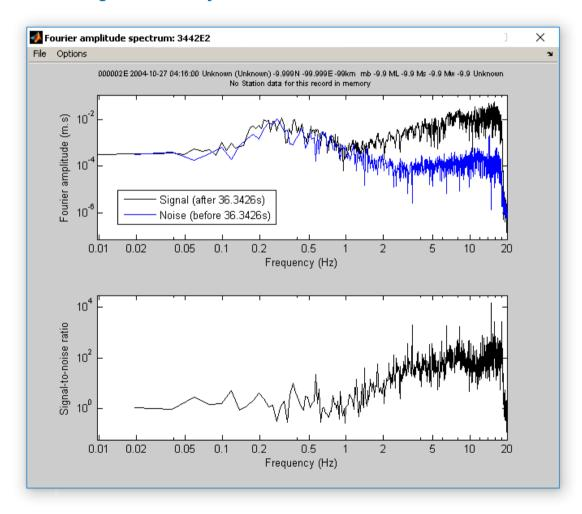
Clicking on this button when a single time-history has been selected will calculate and display the Fourier amplitude spectrum of the currently selected time-history. No smoothing of the Fourier amplitude spectrum is applied. Two Fourier amplitude
