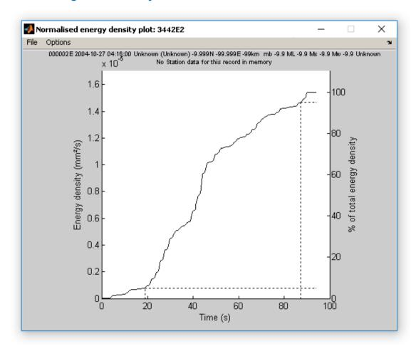
Clicking on this button will calculate and display the normalized energy density plot [i.e. energy density against time (Sarma, 1971)] of the currently selected time-history. The left hand axis gives the normalized energy density [note that, to get the true energy density, the normalized energy density should be multiplied by Vp/4 where V
